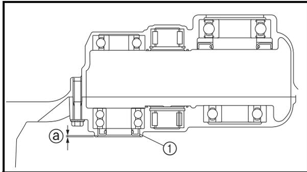
**INSTALLING THE PRIMARY DRIVE GEAR OIL SEAL**
