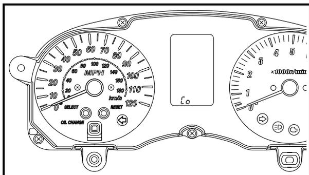
3. Press the “SELECT” button to select the CO adjustment mode “CO” or the diagnostic mode “dIAG”.
