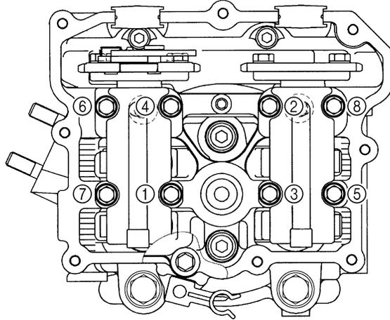
Cylinder head tightening sequence:
