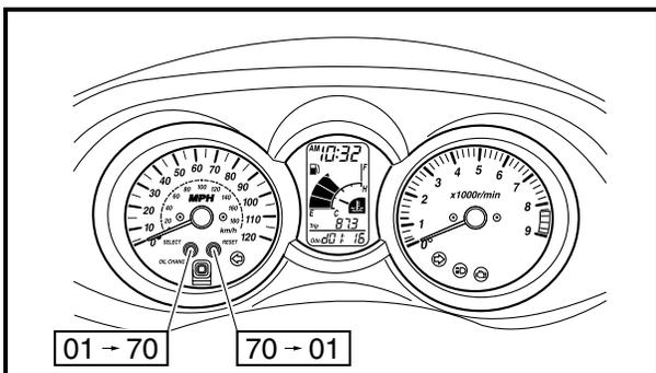
4. Press the "SELECT" button to select the CO adjustment mode "Co" or the diagnostic mode "DIAG".
