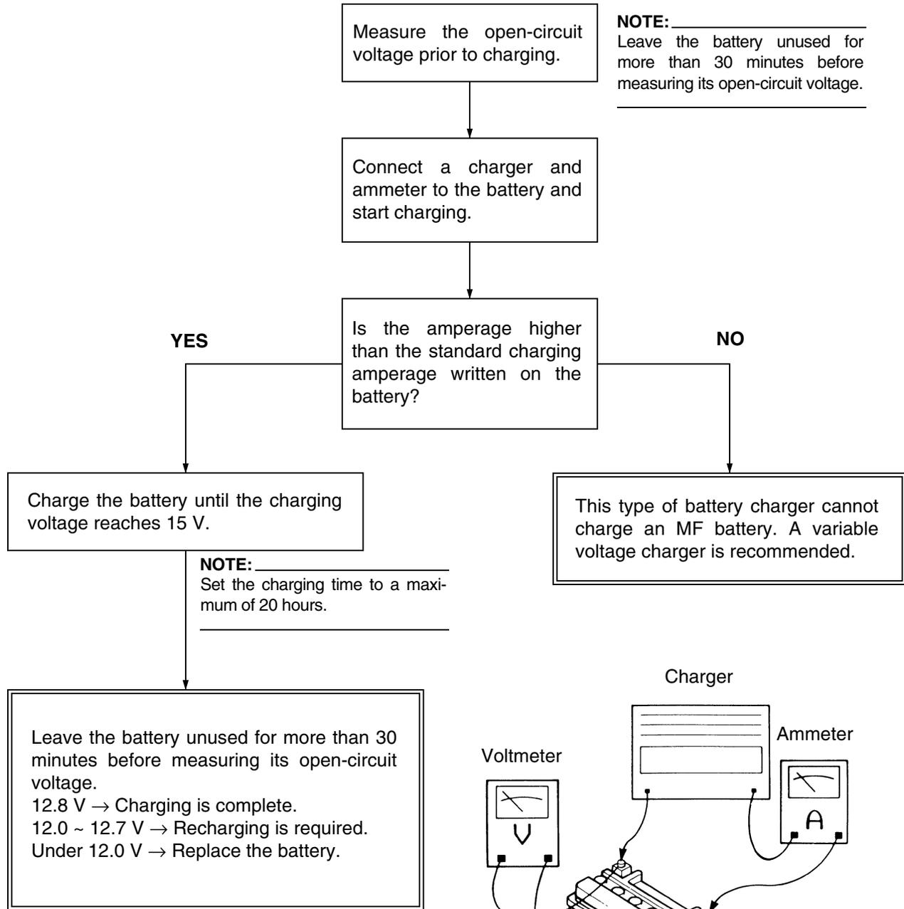
**CAUTION:** Constant amperage chargers are not suitable for charging MF batteries.
