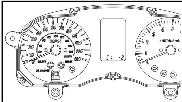
5. Check that “C1” appears on the odometer LCD, and then simultaneously press the “SELECT” and “RESET” buttons for 2 seconds or more.
