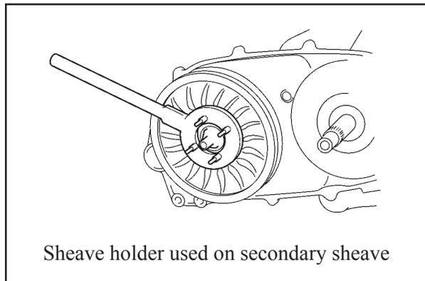
Sheave holder used on secondary sheave
